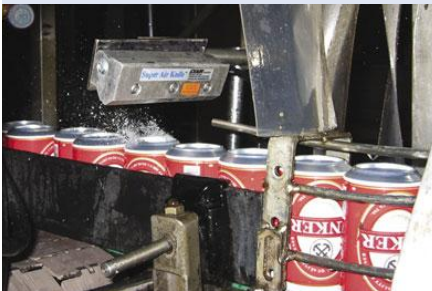
Model 110006 6" (152mm) Super Air Knife removes residual water from can bottoms after a rinse process, eliminating water damage to packaging and shipping materials.
