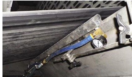
A Model 110048PKI 48" (1219mm) Super Air Knife with Plumbing Kit installed uses EXAIR's Universal Air Knife Mounting System to maintain proper position for removing dust on a conveyor belt and eliminate carryover accumulation.
