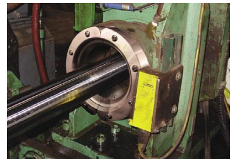
A Model 2404 4" (102mm) Super Air Wipe cleans a steel rod after processing.
