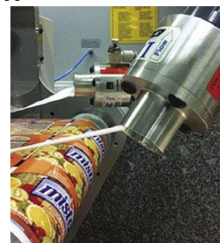
1" (25mm) Line Vacs remove and discard a label matrix.
