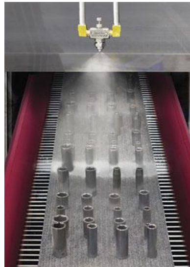
A Model SF1020SS is used to apply a light coating of oil to prevent sockets from rusting prior to a packaging operation.
