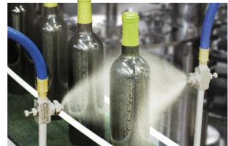
(2) Model EB1030SS atomizing nozzles are used to give a final sanitary rinse prior to labeling wine bottles.
