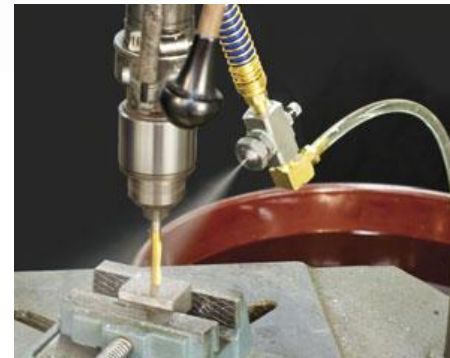
A Model SR1010SS is used to supply a cooling mist for a drilling operation.
