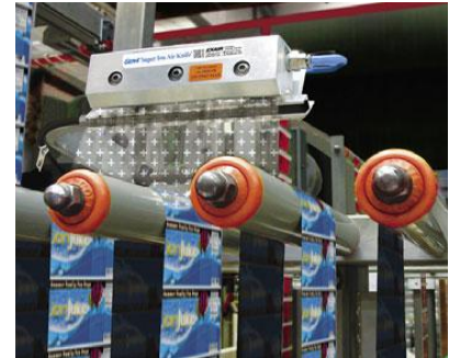
The Gen4 Super Ion Air Knife eliminates the static charge on labels being applied to PET soft drink bottles.
