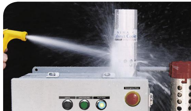
A Model 4830 NEMA 4 Cabinet Cooler cools a panel with 20°F (-7°C) air while keeping the inside dry.
