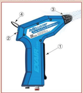
Pressing the full finger, short throw trigger (1) activates the static eliminating ions and airflow. Proper or improper functionality is indicated by a green or red LED (2). The non-marring nozzle (3) provides guiet performance and OSHA compliance. A hanger hook (4) is included to keep the Intellistat conveniently stored.
