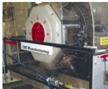
EXAIR's Cold Gun is mounted under the protective guard.
