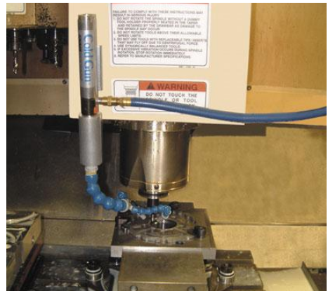
The Model 5315 Cold Gun cools a two flute 3/8" carbide cutter on a CNC, increasing tool life by 50%.
